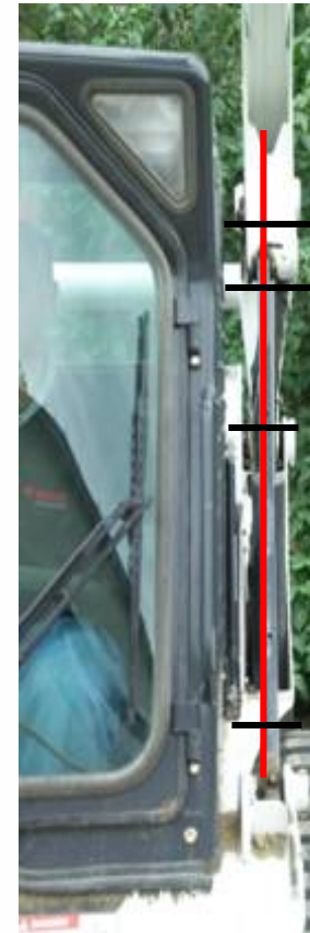
Bobcat pivot pins all in the same plane & are all straddle mounted
